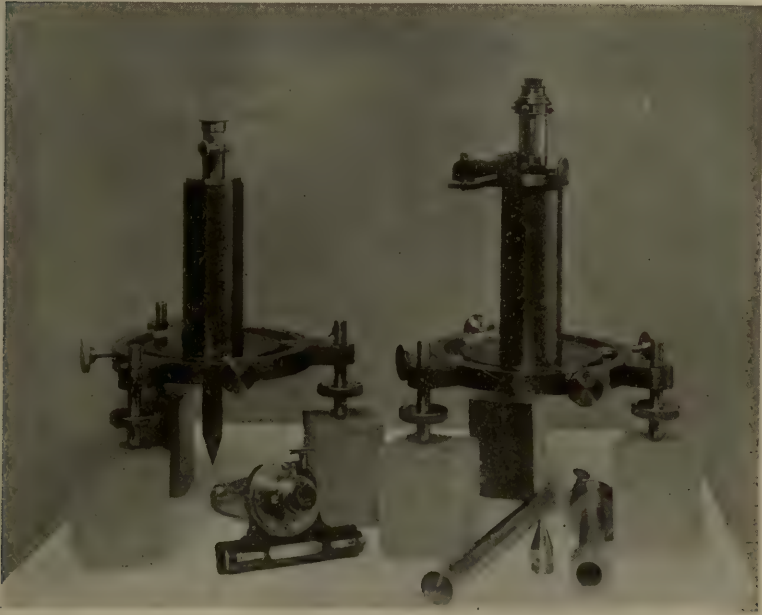
FIG. 30. Vertical Collimator. (Coast and Geodetic Survey.)
